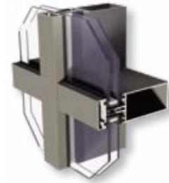
Although the glass used for a curtain wall carries most of the weight when it comes to the final insulation value of the structure, we offer the option of adding extra insulation to the curtain wall profiles. This is why our range includes the **MC PASSIVE** and **MC PASSIVE+** variants. With these variants, Uf values of 1.1 W/m<sup>2</sup>K or 0.97 W/m<sup>2</sup>K respectively can be achieved. Triple glazing can be used; the maximum glass take-up for all versions is 74 mm.
